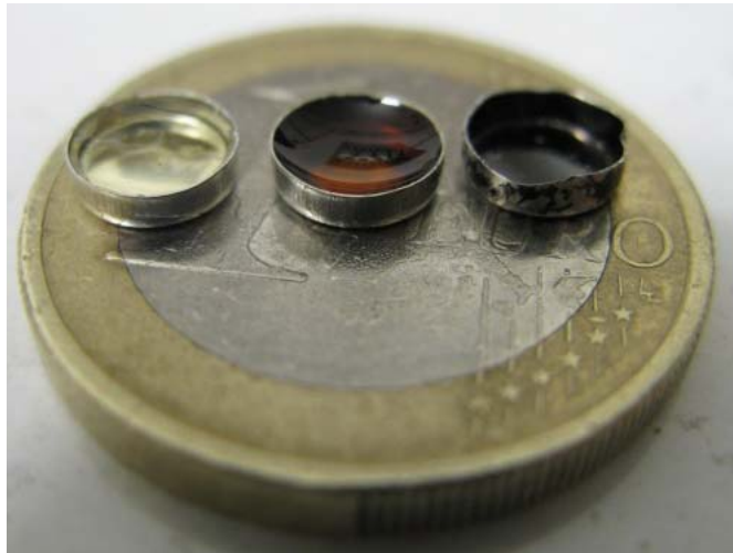
Figure 9. Example of wetting profile of three stages of oil.
